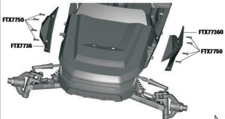
SIDE BODY INSTALLATION B
